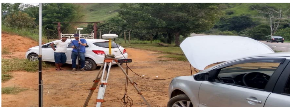
Figura 19 - Receptor RTK na base
