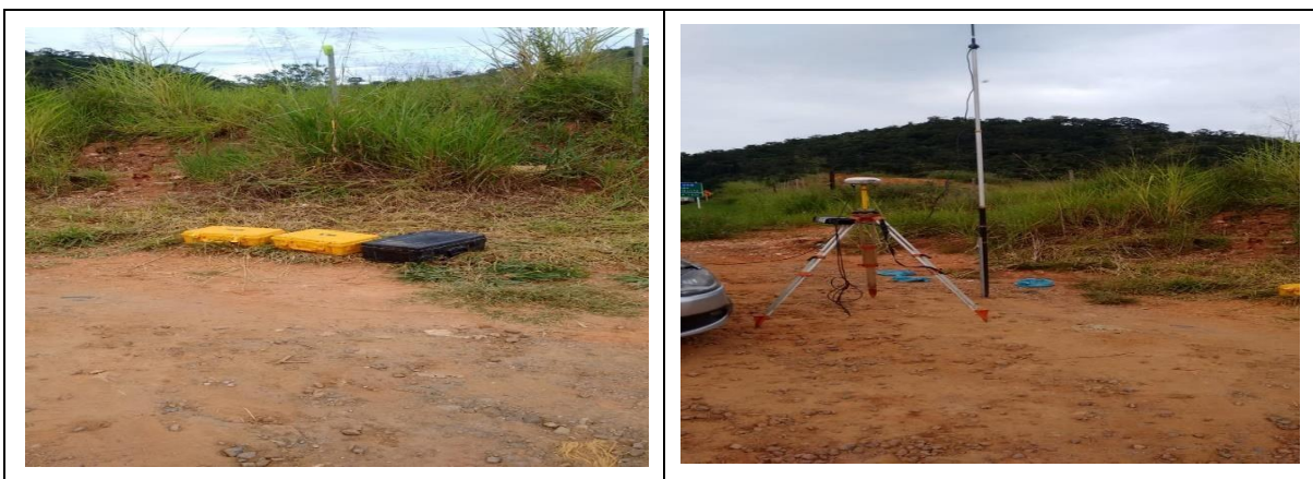
Figura 25 - GPS RTK X 91+ (a) e Receptor instalado na base (b)
